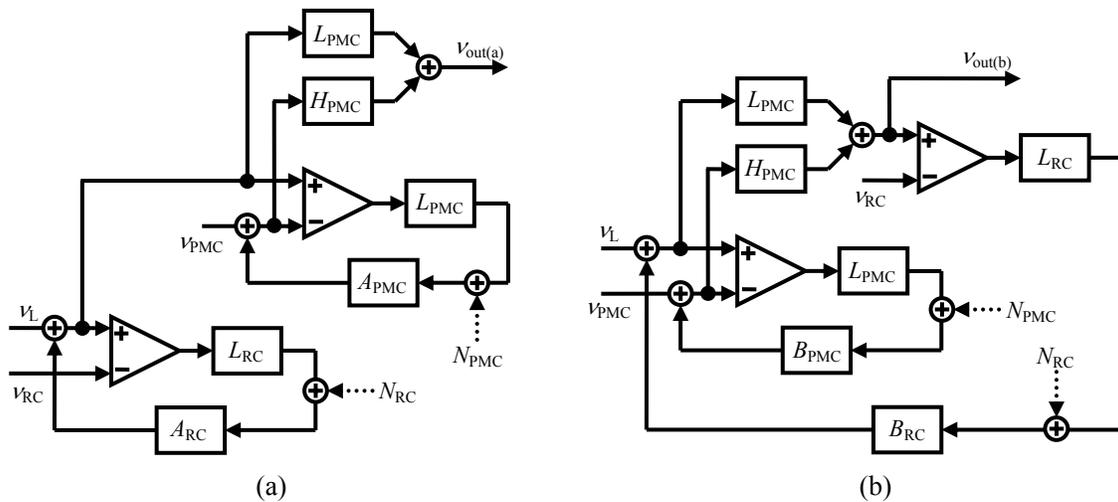
Fig. 3 Noise existing in the cavity servo systems.
