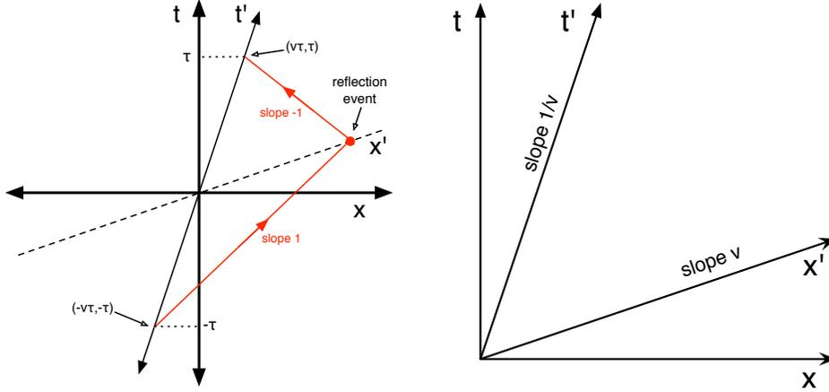
Figure 6: Left: In the  $S$  frame (orthogonal  $(x, t)$  axes), we draw the  $S'$  frame  $(x', t')$  axes; the photon emission, reflection and reception events, and the photon worldlines (with slopes  $\pm 1$ ) that connect them. Right:  $x'$  axis ( $t' = 0$ ) and  $t'$  axis ( $x' = 0$ ) in  $S$  frame space-time diagram.
