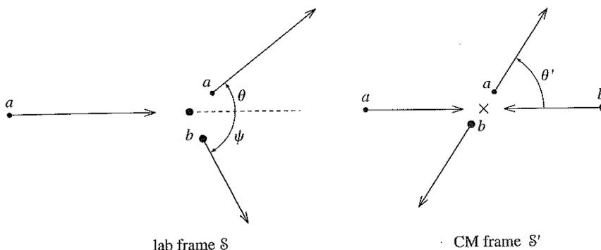
(CM is the center of momentum frame). In the lab frame the incoming particle has energy  $E_a$  and momentum  $\vec{p}_a$ .
