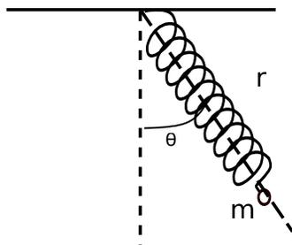
A massless spring with rest length  $l_0$  (with no tension) and stiffness  $k$  hangs in the gravity field. It has a point mass  $m$  connected to one end and the other end fixed. The motion of the system is only in one vertical plane (the plane of the paper).
