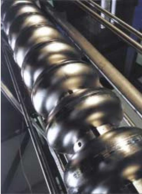
**TESLA Superconducting Cavity**
