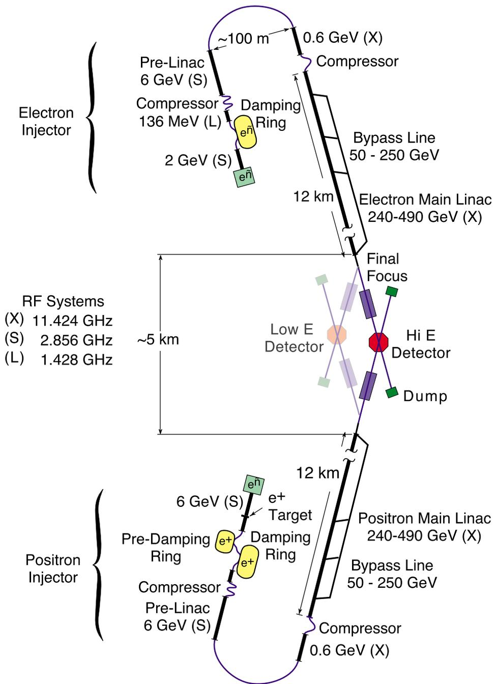
**Figure 4.1. The NLC. The schematic drawing illustrates the elements of a linear collider. In one model of international organization, different countries could supply different parts of the project. From this point of view, TESLA and JLC are similar to the NLC.**
